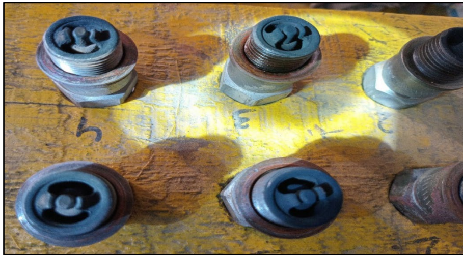
Figure 3 Heavy carbon deposits observed on electrodes
