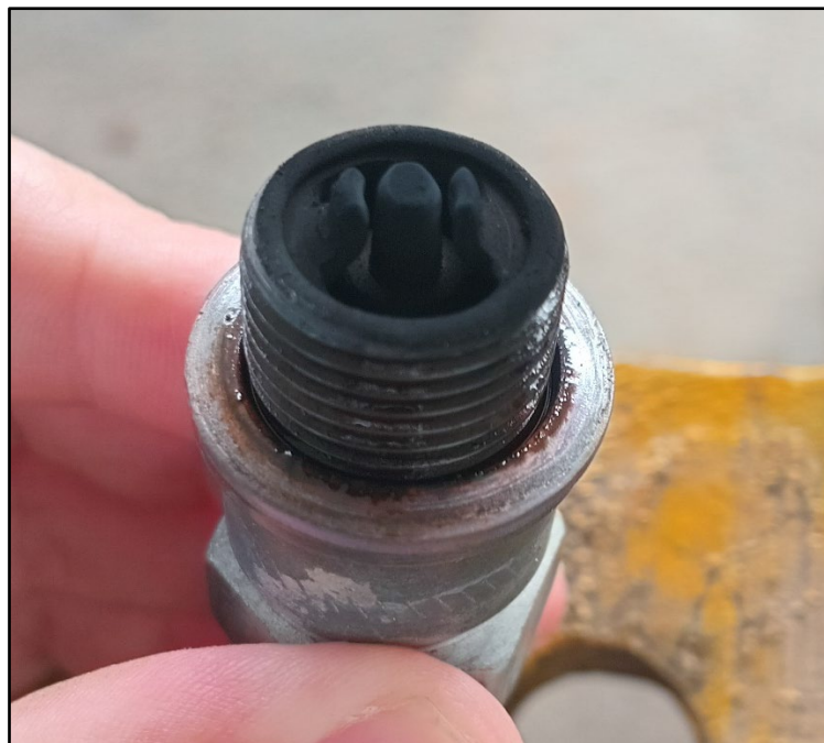
Figure 6 Oil deposits observed on the electrode ends
