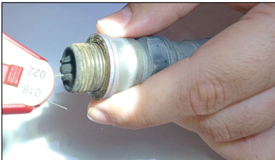
Figure 4 Gaps exceeding OEM-specified limits
