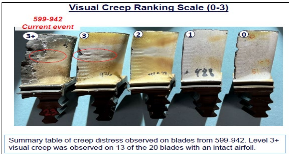
Figure 5 Creep Distress observed on Blades
