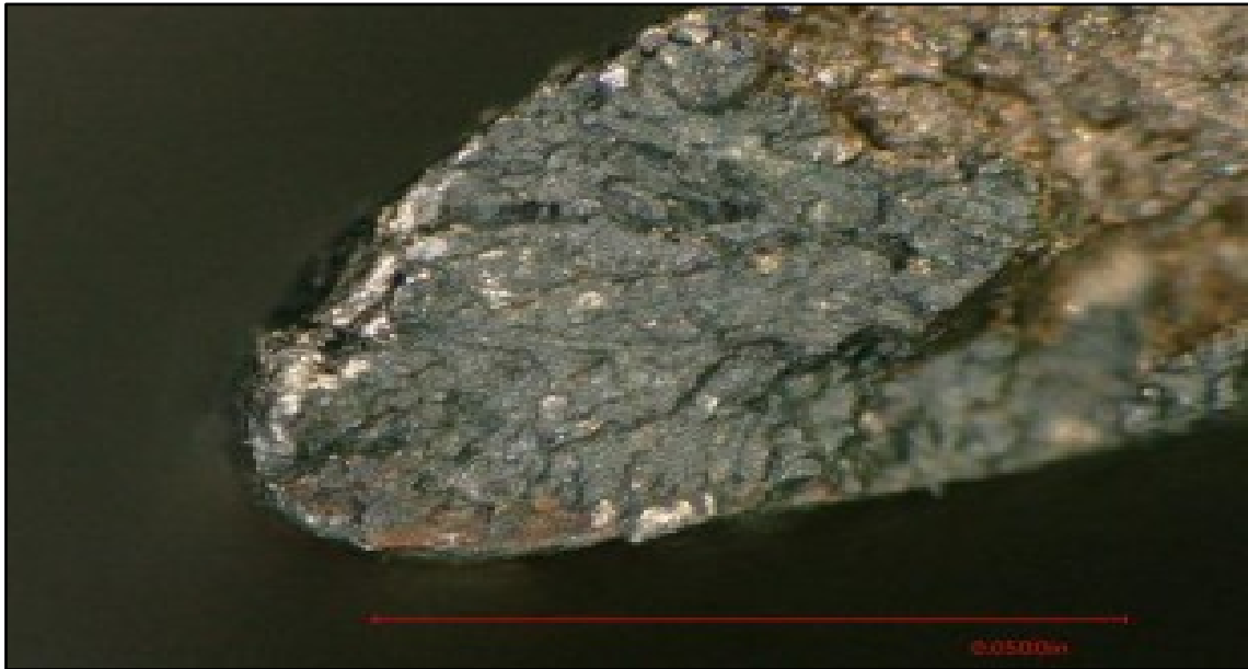
Figure 17 Magnified view of the blade No. 50 fracture surface
